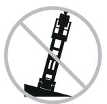
Do not depend on the tilt alarm as a level indicator. The tilt alarm sounds on the chassis only when the machine is on a slope.
